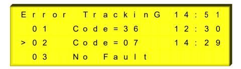
Faults are shown by order on the first viewing screen with their codes and times of occurence. They can be viewed with up and down buttons. When pressed ENTER button, detailed fault information that is shown with the arrow on the left side is screened.
