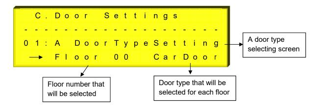
If floor door type is required to change, it is pressed ENTER button second time and lightened right arrow and door type is selected.
