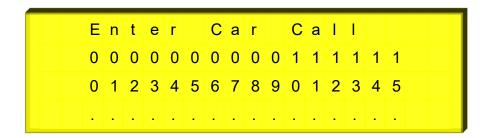
Dots on the screen indicate floor numbers in order. Floor that will be given call is selected with cursor and put "+" sign with "ENTER" on the floor number. More than one call, the other floors are selected the same.
