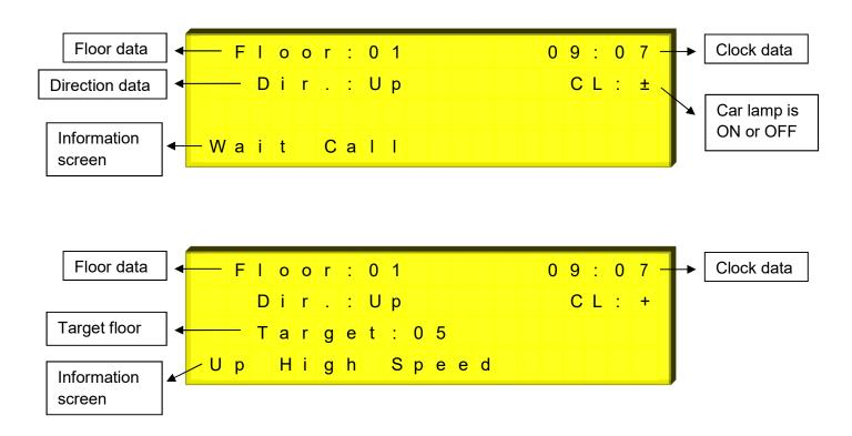
When the car is moving, on the left side of LCD third line, there is target floor.
