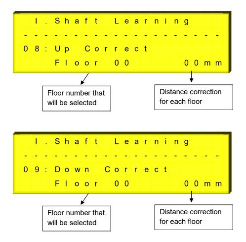
For each floor in shaft learning, at the situation of the car doesn't stop the floor level, it is used for accuracy correction. To enter the parameter, floor is selected with the arrow on left side by pressing ENTER button and by pressing again, distance correction is done as (-) or (+) value with arrow on the right side. Distances are indicated one by one or by using "For All" option in the left side of parameter, the same correction for all floors can be entered.
