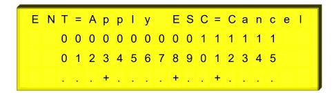
On the screen, registrations are canceled with "ESC" button or registrations are confirmed with "ENTER" button and exit from the function.
