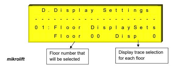
It is used for trace type selection that is required to be traced on floor for every floor. To change the parameter; first, by pressing ENTER button, floor is selected with arrow on left side. By pressing ENTER button again, display that will be traced is adjusted with arrow on right side.
