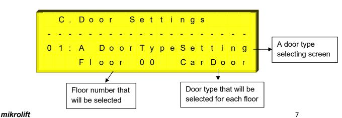
For selection, with lightening left arrow by pressing ENTER button, required floor is selected.
