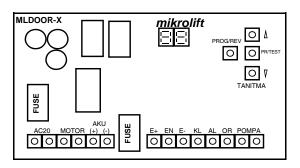
AC20 Transformer Input,60...90VA 0-20 Volt 24 V DC Motor 12 V 1.2 Ah Dry Battery AKU E+ Encoder (+) ΕN Encoder Encoder (-) Close Limit (Open when door closed) Open Limit (Open when door open) OR Limit Common
